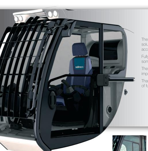
The ergonomic H-cab model embraces the operator. A unique solution in this category (1050 mm /41.6 in wide) in which several accessories facilitate the work of the operator.
