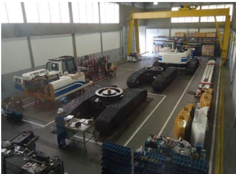
Production line of the Soilmec SR-55 on a Caterpillar turret.
